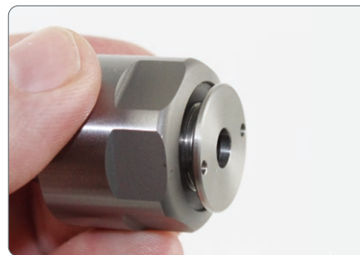
1. Thread coolant cap into SXCN nut, tighten with wrench after the collet has been assembled.
